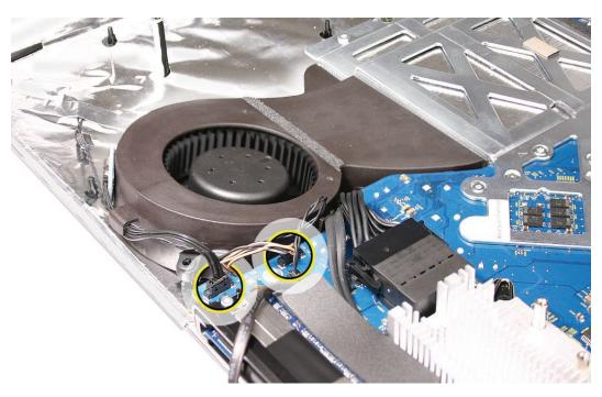
2. Disconnect the cable from the sensor board on the speaker.
